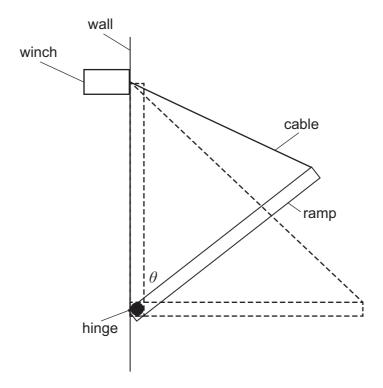
The ramp is lowered slowly, at constant speed, from its closed (vertical) position ( $\theta = 0^{\circ}$ ) to its open (horizontal) position ( $\theta = 90^{\circ}$ ).
