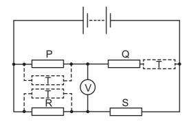
Which of the positions for resistor T causes an increase in the magnitude of the voltmeter reading?
