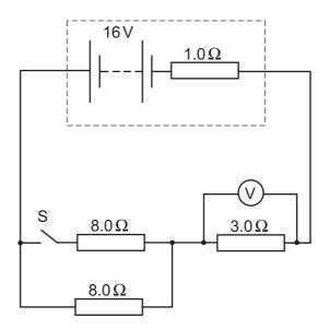
Which line in the table gives the voltmeter readings when switch S is in its open and closed states?
